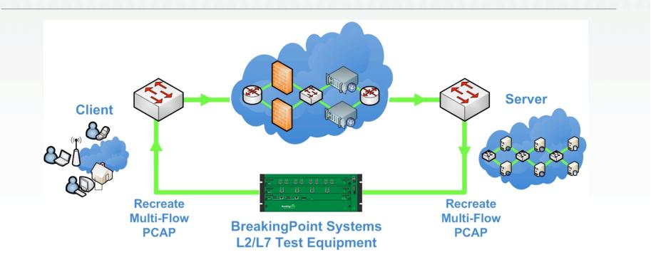
The BreakingPoint Recreate feature recreates multi-flow TCP/ UDP traffic based on data from PCAP. BreakingPoint does not use a raw playback, instead it will do stateful multi-flow allowing possibility to replay stateful TCP/UDP traffic with ability to amplify.
