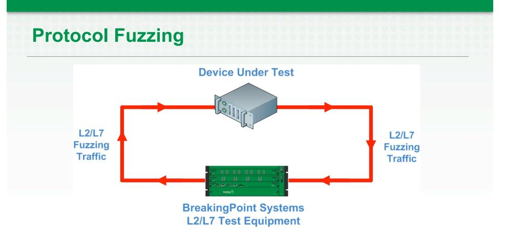
Stack Scrambler tests the integrity of different protocol stacks by sending malformed packets to the device under test. It uses a fuzzing technique, which modifies a part of the packet (checksum, protocol options, etc.) to generate the corrupt data.
