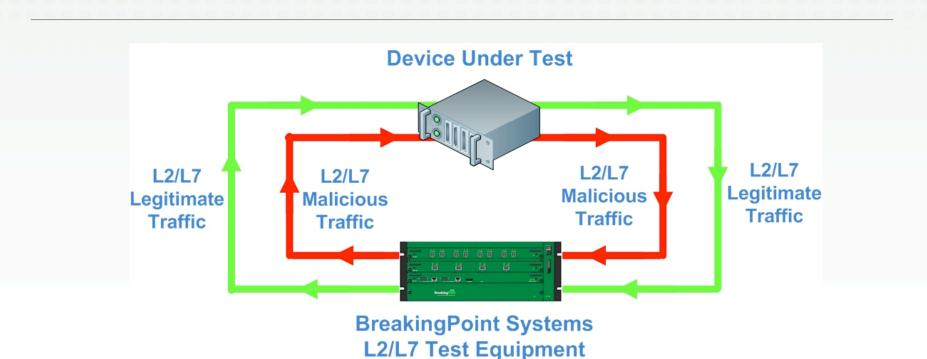
BreakingPoint properly tests high-performance security devices with the capability to mix good traffic and malicious traffic emulating real world test scenarios.
