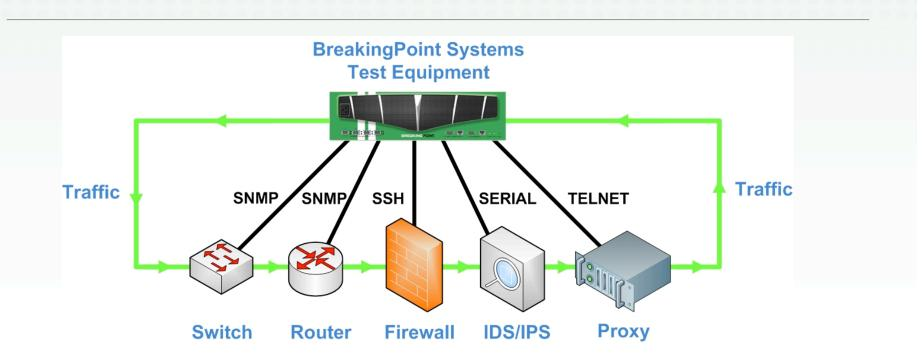
BreakingPoint offers the ability to connect to a DUT via Telnet, SNMP, SSH, or Serial to monitor the status of a DUT offering the ability to check CPU, Memory, New TCP connections per Second, Concurrent TCP Connections, Bandwidth and Packet per Second. Eliminates manual power-cycle reboots.
